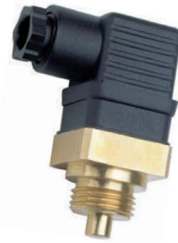
The bimetal thermostat built into the compact housing switches upon reaching the limit temperature. The contact is available as either NC or NO. It can be installed at any position and is mounted preferably in the place of an oil drain screw or one of the oil sight glasses.
