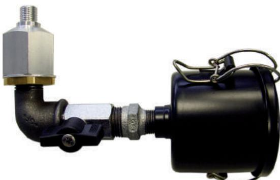
Gas ballast valves prevent condensing vapours from contaminating the pump oil. The oil-water emulsion arising from contamination reduces the pump efficiency or leads to a failure. The valve permits a regulated amount of fresh air (the gas ballast) to flow into the pump's compression chamber. By mixing saturated intake air with unsaturated fresh air, condensing is suppressed.
